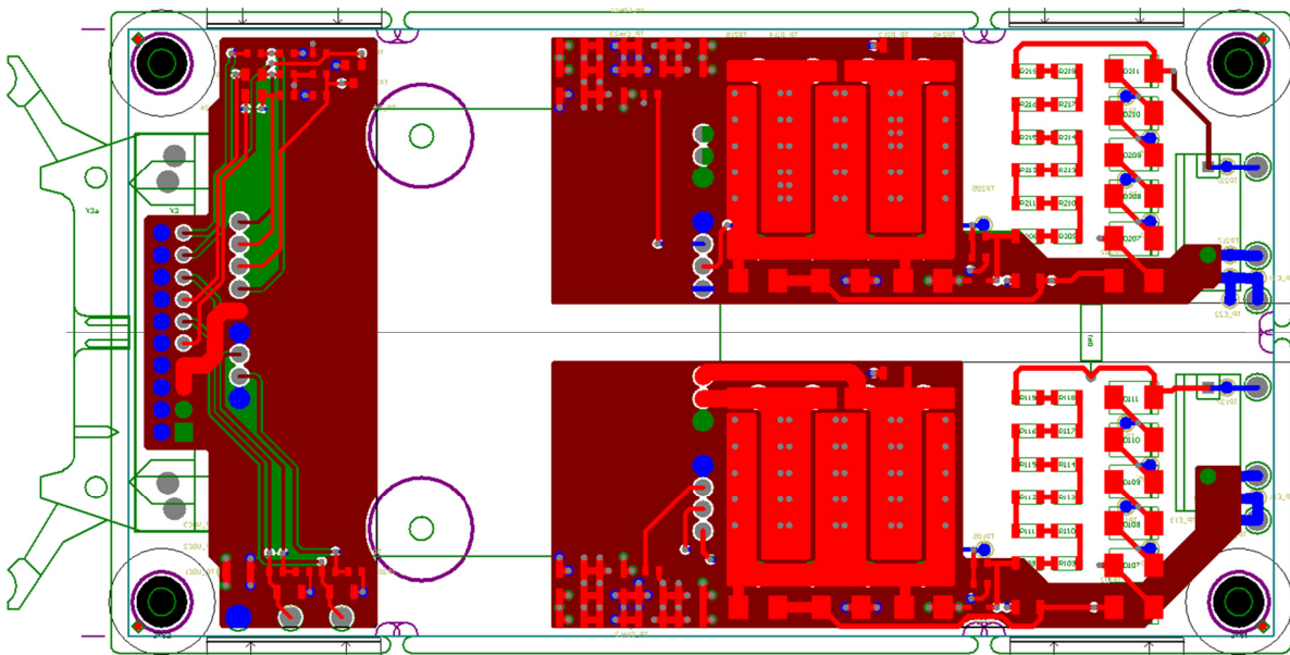
Fig. 27 PCB layout of CONCEPT base board 2BB0435T
